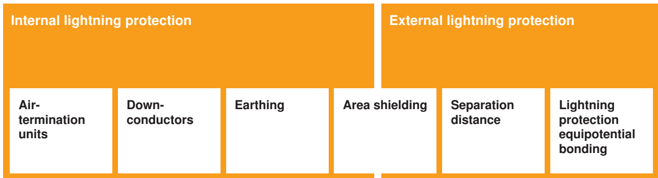
External and internal lightning protection systems
