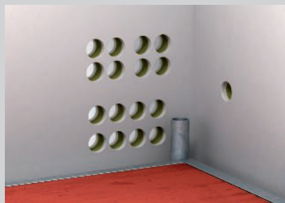
Grouped arrangement of the drill holes.
