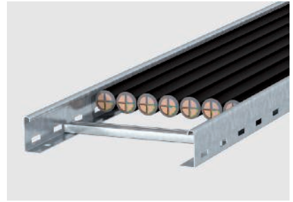
Cable ladders for power cables with a large cross-section Areas of application: Cables and power conductors with large cross-sections. These can be fastened to the rungs using clamp clips. The high load capacity and good ventilation ensure perfect cable laying.
