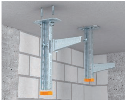
Standard mounting of suspended support with wall bracket, single-sided without spacer Ceiling fastening of a suspended support with single-sided bracket fastening. A spacer is not always required for widths up to and including 300 mm.
