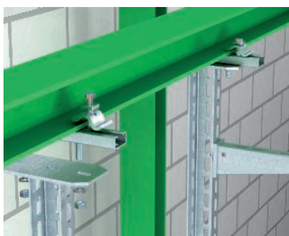
Clamp fastening with addition C profile Use of an additional C profile rail, type MS, for wider steel girders. Route along steel girder.
