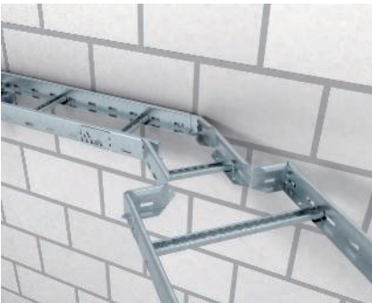
Multifunctional connector for cable ladders Creation of a reduction, including 45° angle, using a multifunctional connector, type LMFV.
