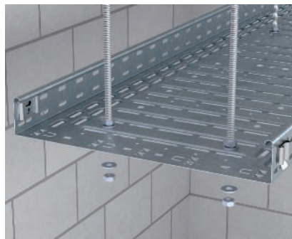
Threaded rod suspension RKSM > 400 mm The threaded rod suspension of RKSM cable trays > 400 mm can take place using two threaded rods.
