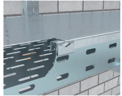
Screwless cover mounting Unperforated covers are mounted using cover clamps, type DK DRLU. The cover clamps are first clamped to the cover edge and then snapped on to the cable tray rail with the cover.
