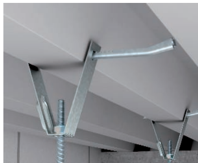
Installation of trapeze suspension Installation of a cable tray on a trapezoidal ceiling using a ceiling bracket, type TPB 100 and centre suspension, type MAH 60. Maximum cable tray width 300 mm. The trapezoidal fastening is mounted using the lock, type TPB R.
