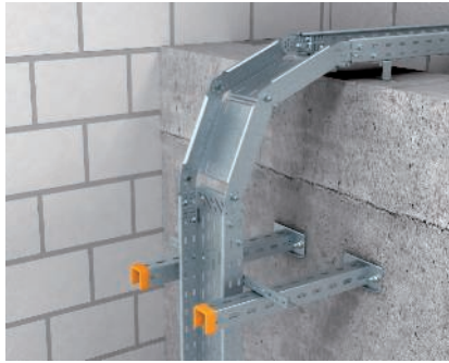
Installation of falling adjustable vertical bend Adjustable vertical bend to bridge height offsets. The adjustable vertical bend is connected with to the cable tray using the adjustable connectors.
