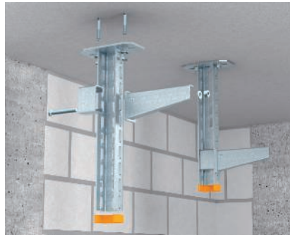
Standard mounting of support with wall and support bracket, single-sided with spacer Cover fixing of a suspended support with single-sided bracket fixing. For widths of over 400 mm, we recommend using a spacer.
