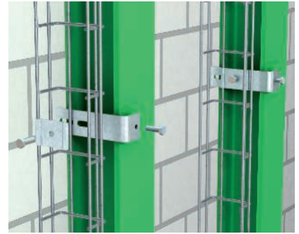
Vertical clamp fastening Installation of a mesh cable tray vertically on a steel girder, mounting with a beam clamp BFK and clamp GKS 50.
