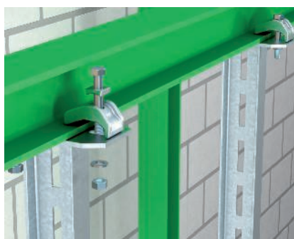
Direct girder clamping Direct girder clamping of an I suspended support using chuck jaw (heavy duty), type TKS-S-30. Route along steel girder.
