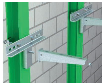
Clamp fastening on vertical steel girder Mounting of the adapter plate, type KA-AW, on the vertical steel girder using clamping angles or chuck jaws. Wall brackets of type AW are fastened to the adapter plate, using the hexagon head screw SKS 12x40 GF.
