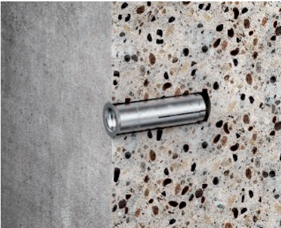
Drop-in anchor, type ES Impact tie, type E, with M6, M8, M10, M12 internal thread. To accept small loads, approved for multiple fixings in cracked and non-cracked concrete of non-load-bearing systems.
