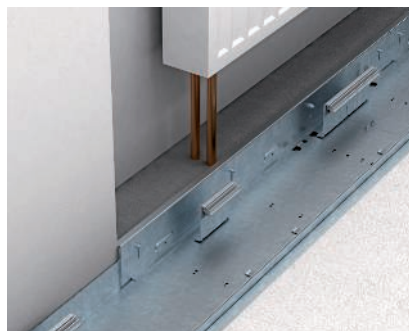
Use of the screed limitation profile When the screed is laid on both sides, mount the screed limitation profile on the wall side of the trunking system.
