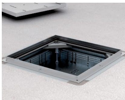
Mounting of lid heavy-duty support Insert the four heavy-duty lid supports in the corners of the underfloor box and adjust them to the required height. Lock the support screw with a locknut.
