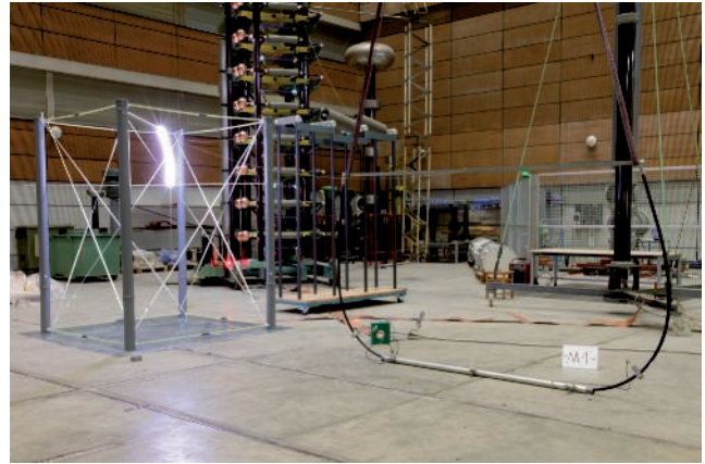
Testing structure during an impulse voltage test with an equivalent separation distance ( s_e ) of 75 cm.
