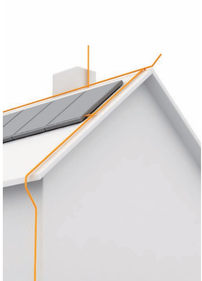
Direct connection of PV mounting frames to the lightning protection down-conductor system
