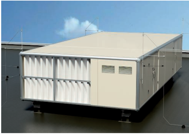
Insulated air-termination system with separation distance (s)
